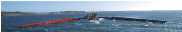
Fig. 12 Wave dragon overtopping WEC
