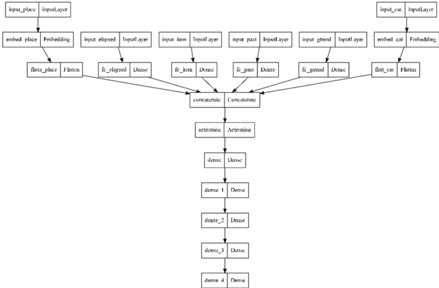
Fig. 5. DNN model with entity embedding
