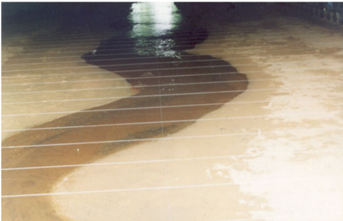
Fig. 1 View of the experimental alluvial channel
