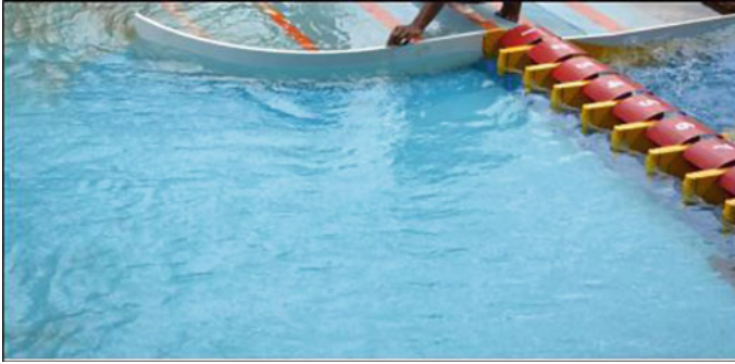
Photo 6 Flow conditions after modifying upstream curved guide wall with full curve height upto dam Top El. 244.955 m
