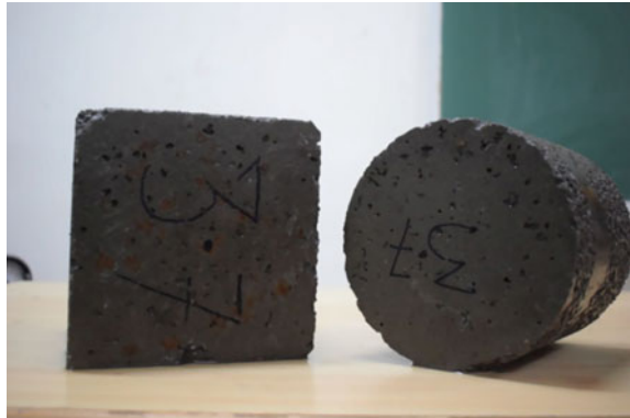
Fig. 4 Specimen showing cement paste drain at the bottom
