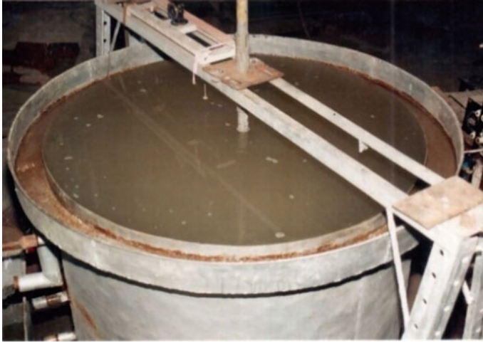
Fig. 1 View of experimental setup used for scour studies
