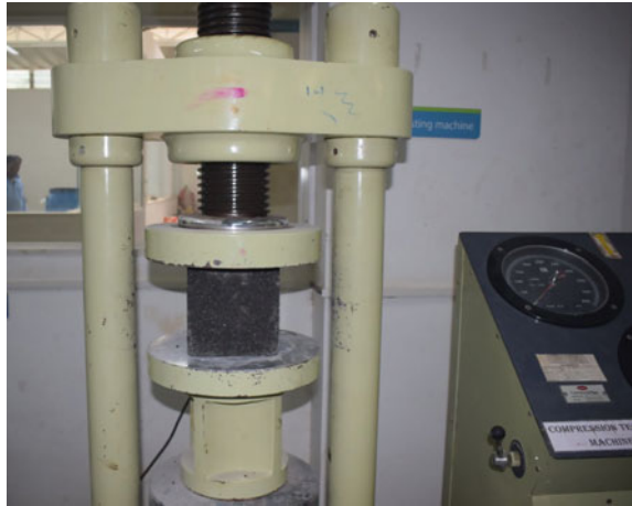
Fig. 7 Compressive testing of pervious concrete specimen
