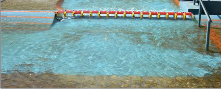
Photo 2 Upstream flow condition of spillway for Q = 24,131 \text{ m}^3/\text{s} for ungated operation of spillway
