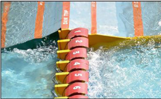
Photo 3 Intermixing of flow due to abrupt change in the direction of flow for Q = 24,131 \text{ m}^3/\text{s} for ungated operation of spillway
