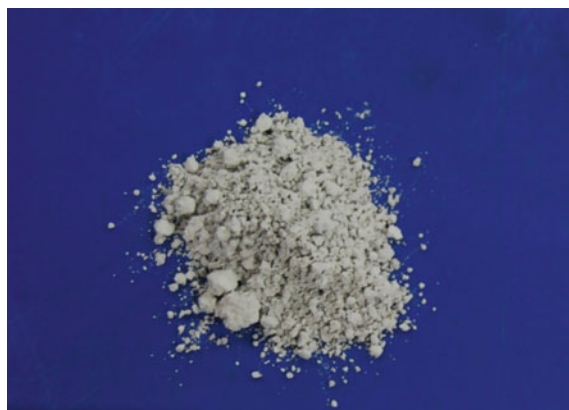
Fig. 3 Micro GGBS (Ground granulated blast slag)
