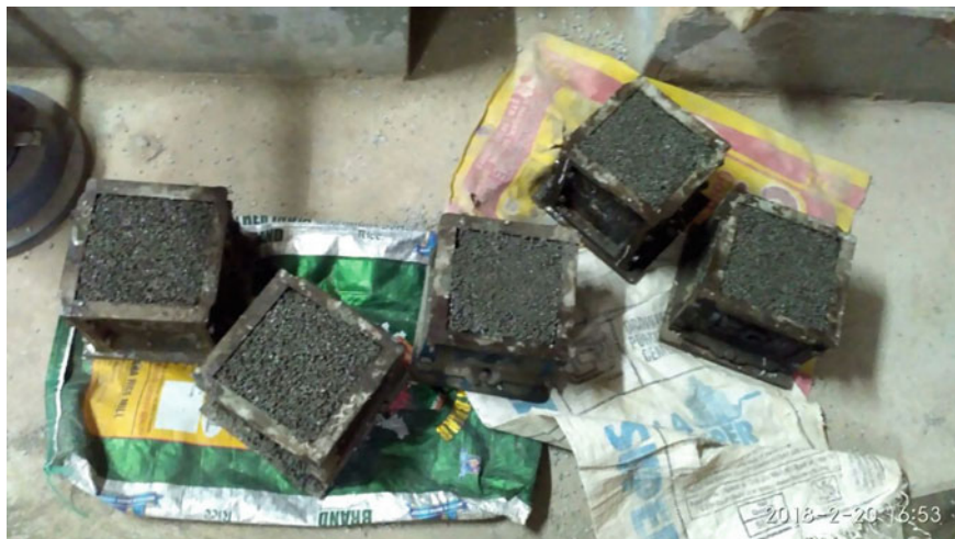
Fig. 5. 150 mm × 150 mm × 150 mm specimen for compressive strength
