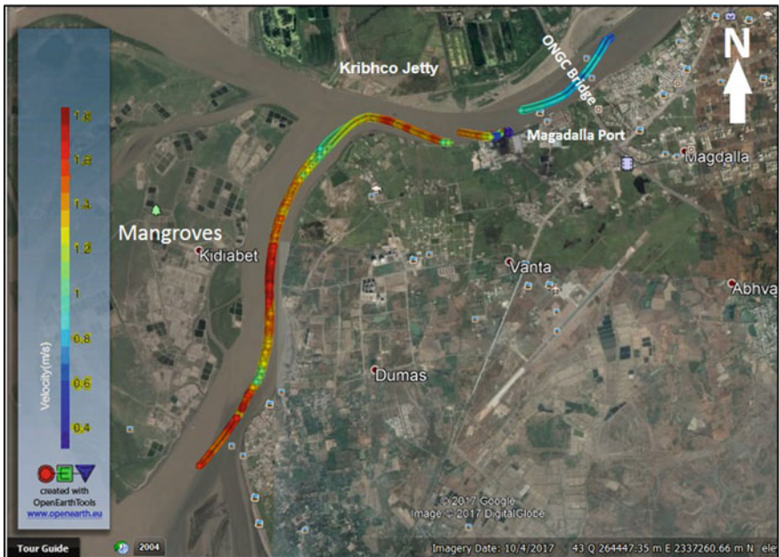
Fig. 8 Measured GPS drifter trajectories
