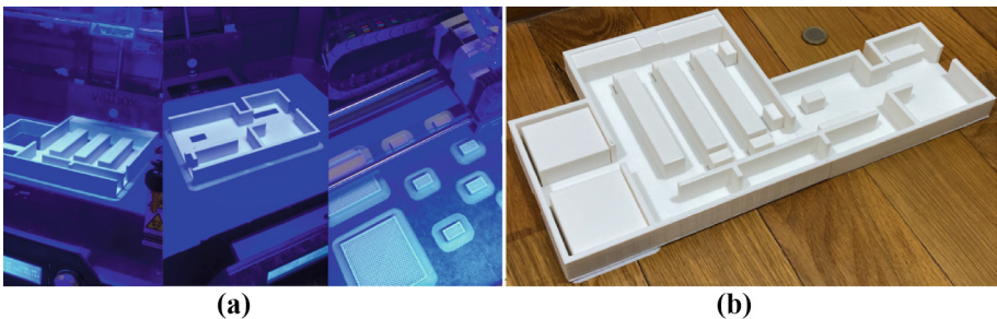
Fig. 4. From left to right: a) Illustrative photos of the 3D printing process; b) The 3D interior layout plan of the museum.
