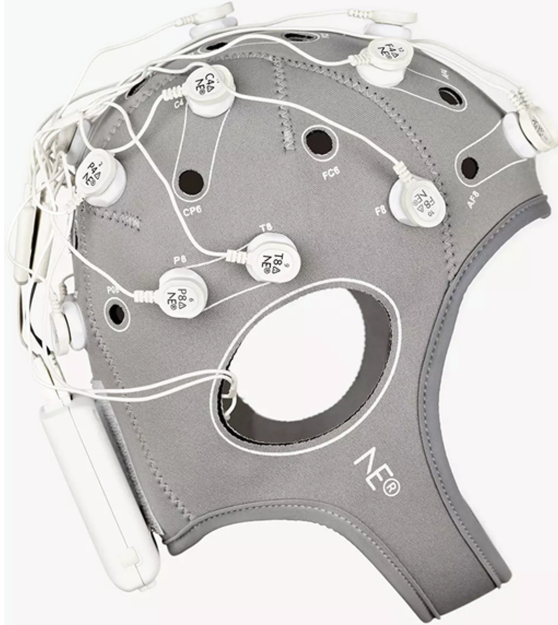
Fig. 2. The Enobio brain computer interface headset.
