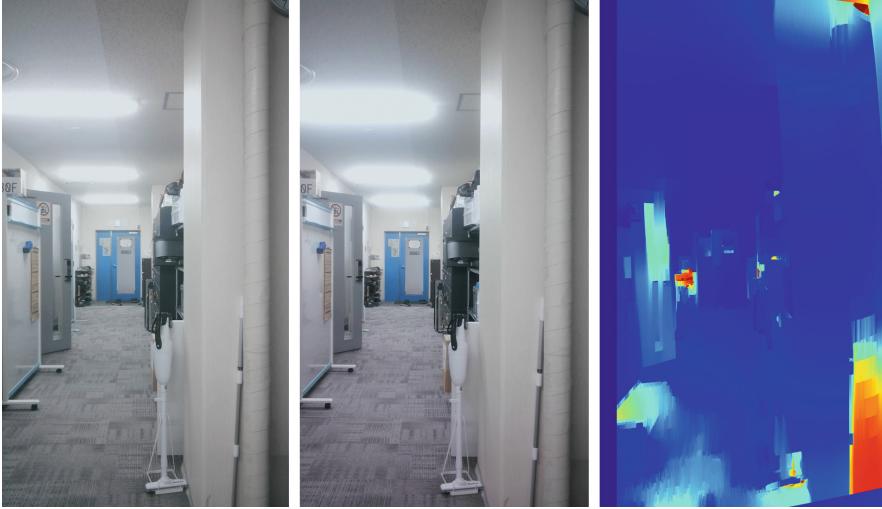
Fig. 5. A sample of left view, right view, and depth map of the stereo vision system we build. The miscalculation on the shoe shelf in the middle left of the view can be observed.
