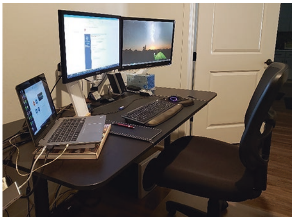
Fig. 1.7 Ergonomic work station with laptop elevated so it is at eye level to prevent neck strain and an adjustable chair
