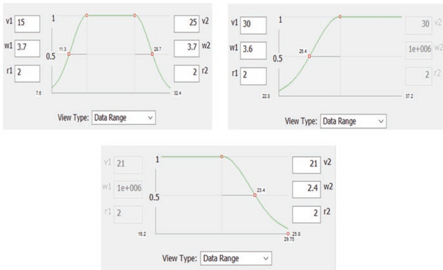
Fig. 10.2 Examples of the bell-shape, S-shape, and Z-shape optimality curves utilized in the ArcSIE inference interface
