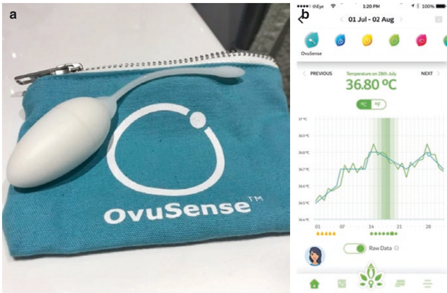
Fig. 5.6 The Ovusense sensor designed to track menstrual cycle using Core Body Temperature (a) and a screen designed to convey information extracted from the sensor in the Nabta app (b)
