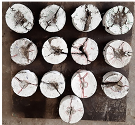
Fig. 11. Impact energy of final failed specimen.
