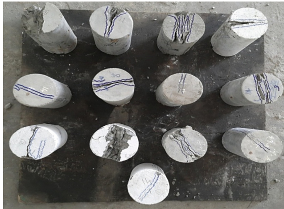
Fig. 9. Final failure specimen of split tensile strength.
