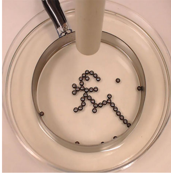
Fig. 4.6 The E-SOFI. Electrically charged beads aggregate into a branching “tree” that serves as a pathway for conducting charges to ground
