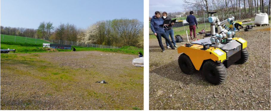
Fig. 3. Left: Deployment of the SNIFFBOT IRC and its WSN in the field. Right: Modified Warthog land robot for tele-inspection and tele-manipulation.
