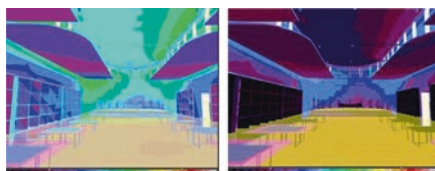
Fig. 9 New lighting proposal: Illuminance (left; lx) and luminance (right; cd/m 2 ) at 10 am – only natural light (artificial light off) for the functional library scenario design
