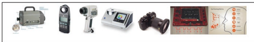
Fig. 1 Some basic instruments for experimental measurements: from left to right, photoradiometer, luxmeter, luminance meter, colorimeter, digital camera with V_\lambda filter, hardware platform Arduino, fundamentals of eye tracker technique
