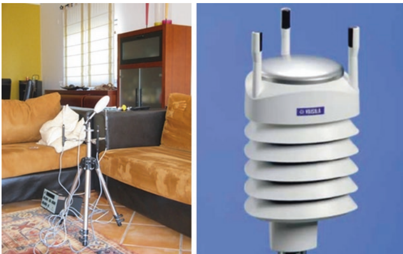
Fig. 2 Thermal comfort assessment equipment and weather station
