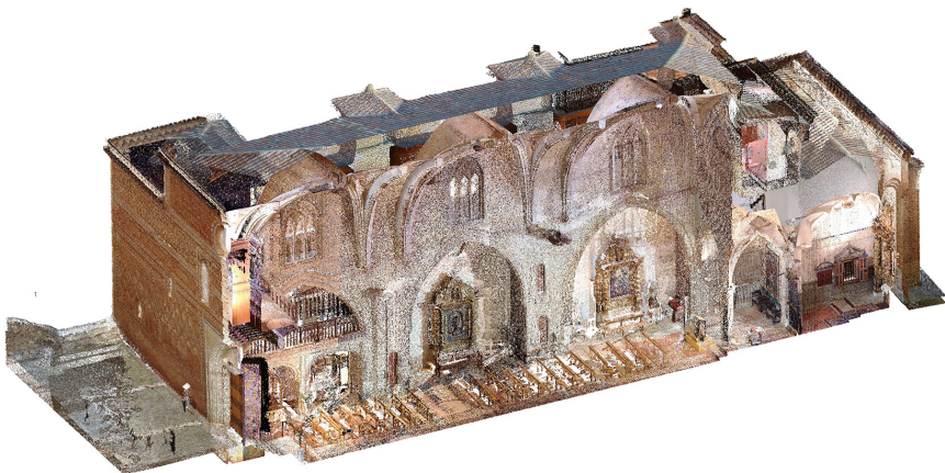
Fig. 1. Complete point cloud of Santa María de Tobed (Prepared by the authors).
