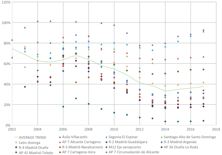
Fig. 2 Yearly traffic deviations (real/expected in %) of the Spanish toll highway concessions since their commissioning. Source: Compiled from Baeza and Vassallo (2012) and updated. Data not available for Santiago–Alto de Santo Domingo from 2014 to 2018
