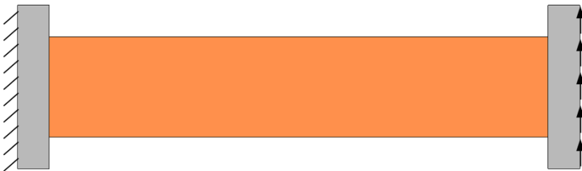
Fig. 16.7 Boundary conditions of computational domain used in the 2nd-gradient theory simulations.
