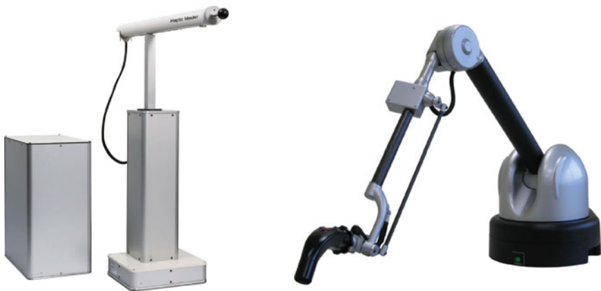
Fig. 6.10 Examples of closed-loop admittance controlled systems in variants with a direct force measurement ( HapticMaster ) and b measurement of the actual current ( Virtuose 6D35-45 ). Images courtesy of Moog FCS , Nieuw-Venep, the Netherlands and Haption GmbH , Aachen, Germany, used with permission
