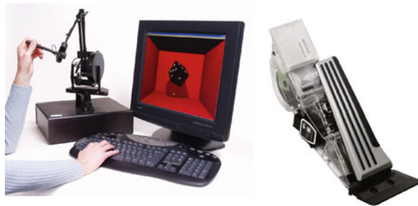
Fig. 2.28 Two haptic interfaces, (PHANTOM PREMIUM 1.5, © 2022 3D Systems geomagic Solutions, Rock Hill, SC, USA) and ACCELERATOR FORCE FEEDBACK PEDAL (AFFP, © 2022 Continental Automotive, Hannover, Germany). Both images used with permission
