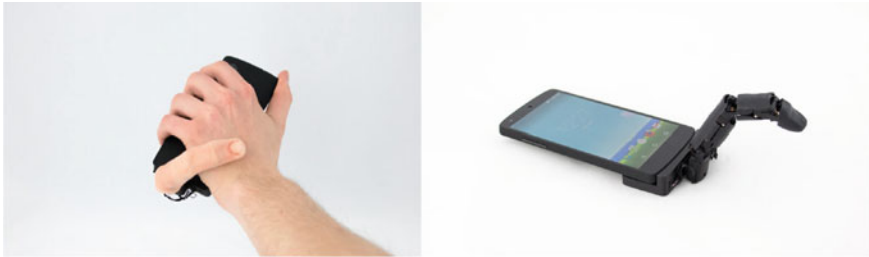
Fig. 1.5 MobiLimb project with a device touching back [11], ©2022 MARC TEYSSIER, used with permission
