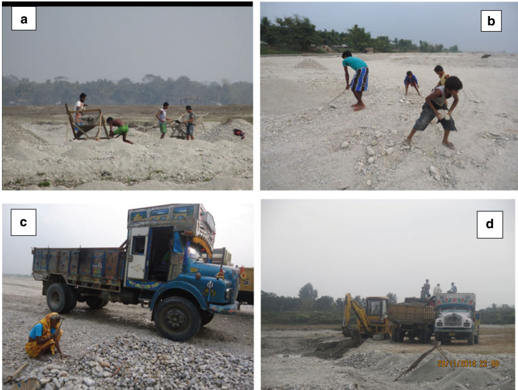
Fig. 2.4 Manual way of sediment extraction wherein crushing, and segregation is done on the riverbed only (a–c); mechanized sediment extractions collect large volume but crushing and segregation happens with sieves at processing units (d)
