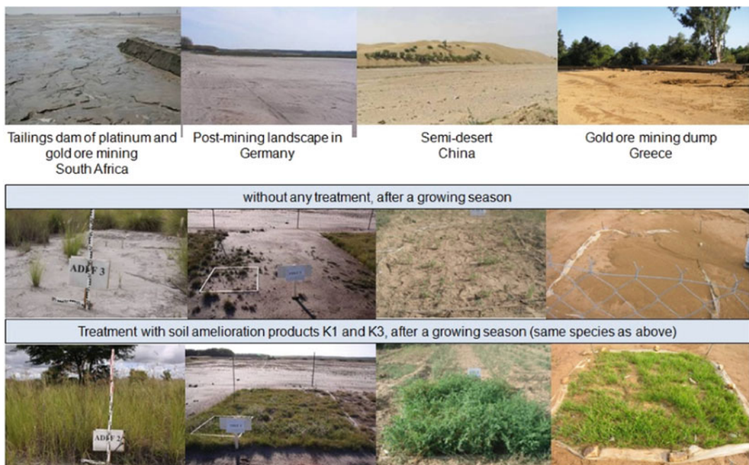
Fig. 16.3 Field trials with K1 and K3 at various extreme locations worldwide
