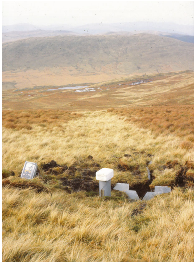
Fig. 11.6 Pipe flow gauging site on Maesnant. Wet grass vegetation follows line of the ephemeral pipe down the hillside
