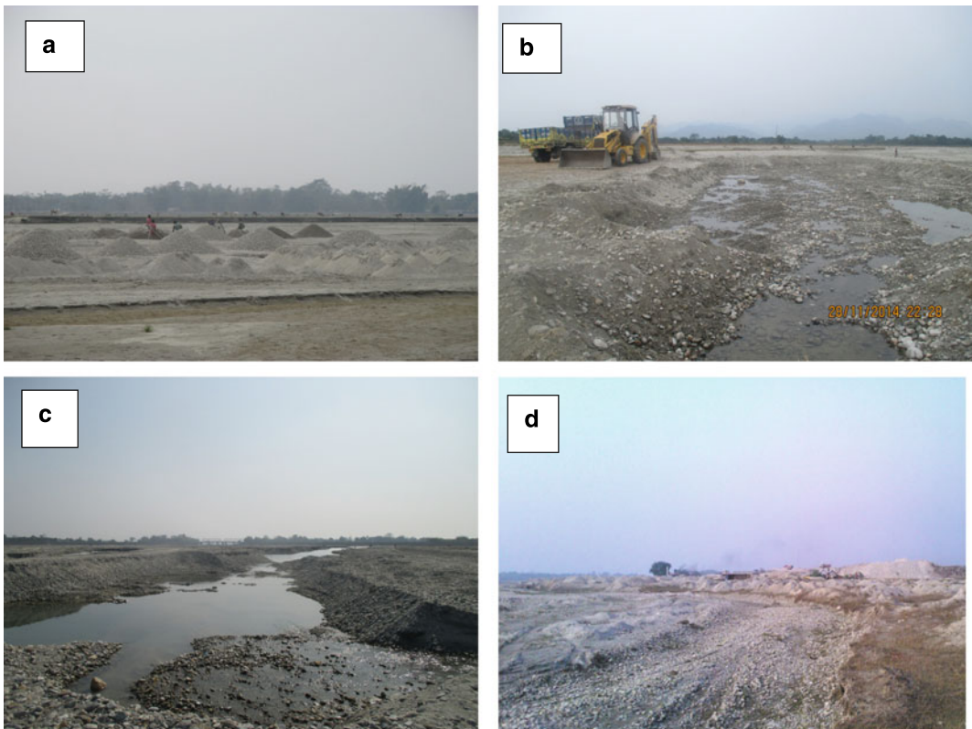
Fig. 2.8 Channel bed deformation due to manual sediment mining (a); mechanized wet-pit mining creating huge longitudinal depressions (negative topography) (b–c); dumping of a huge amount of sediments at Odlabari processing unit creating positive topography of sediment mounds (d)
