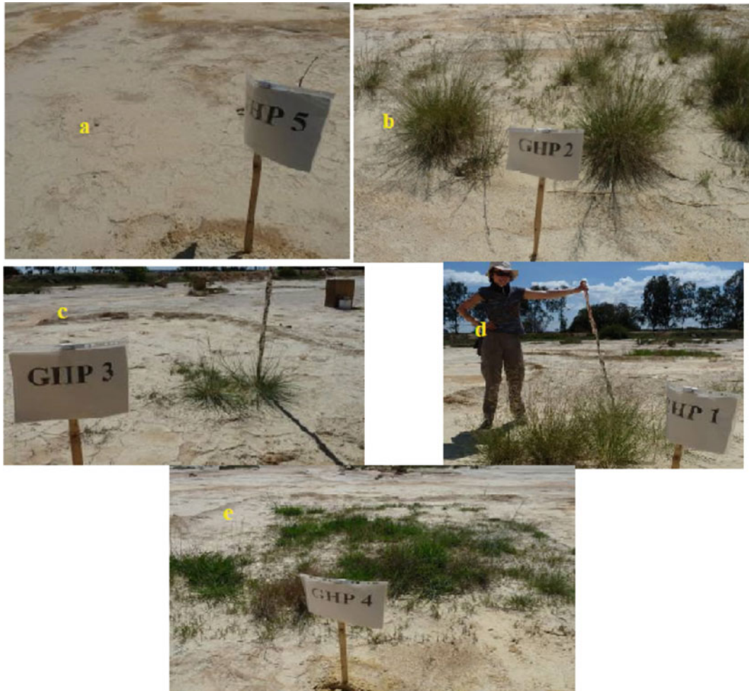
Fig. 16.7 Plant plots on tailings of gold dumps after 3 years; a —Plot with 0% K1 and 0% K3 (Gold 5), b —Plot with 12.5% K3 (Gold 2), c —Plot with 12.5% K1 (Gold 3), d —Plot with 3% K1 and 3% K3 (Gold 1) and e —Plot with 12.5% K1 and 12.5% K3 (Gold 4)
