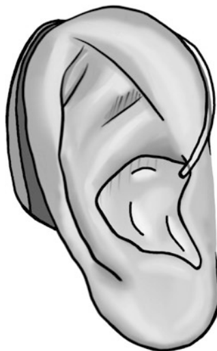
Fig. 16.8 Schematic visualization of a hearing aid including electronic amplifier fixed behind the ear cone, wire for transmitting amplified sounds, and ear piece individually fitted in the ear canal
