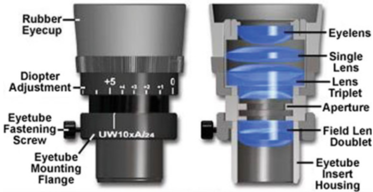
Fig. 2.19 Ultra-wide 10 \times eyepiece with its internal lens system
