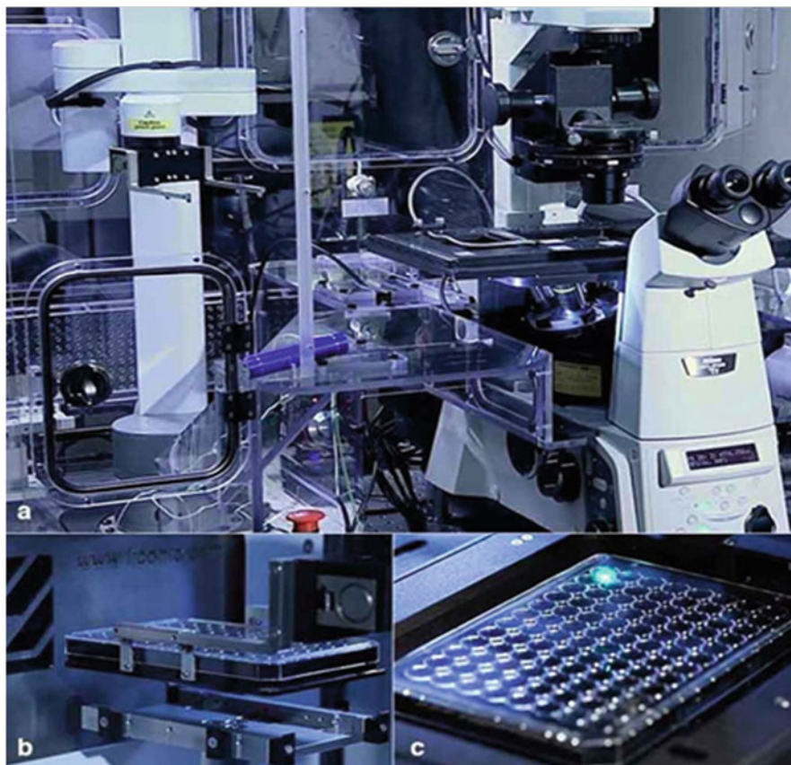
Fig. 6.14 High-content microscope platform based on Nikon Ti-E inverted microscope integrated with a robotic plate loader. Ti2-E can double the throughput of this design (a) for moving samples from incubator (b) to microscope stage (c). The system displayed in this figure belongs to the Finkbeiner laboratory. (Source: https://www.nature.com/articles/nmeth.f.400/figures/1 ) (Reproduced with permission)
