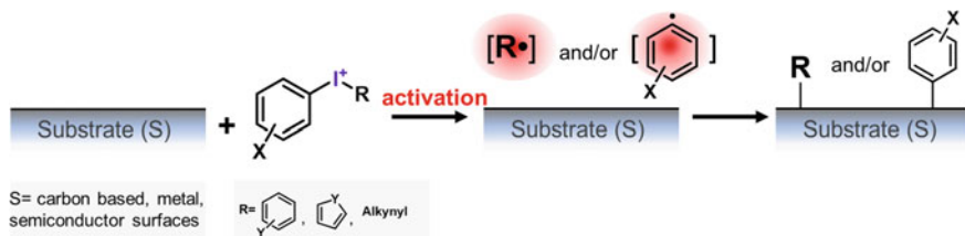
Fig. 2 Principal scheme of surface functionalization using ISs
