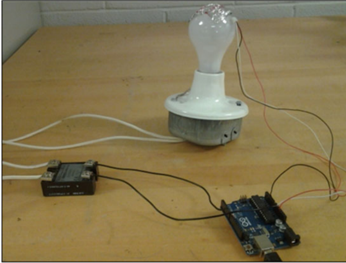
Fig. 1.6 Light bulb, Relay, and Arduino connection scheme. (Source: Mendoza and Cordero (2018))
