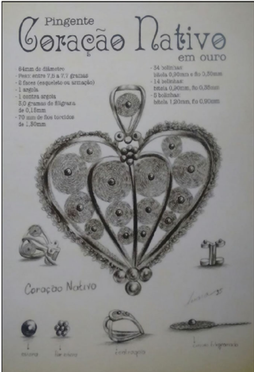
Fig. 6.5 Technical description of the confection of the Native Heart jewelry. (Source: Wall & Araújo, 2015)
