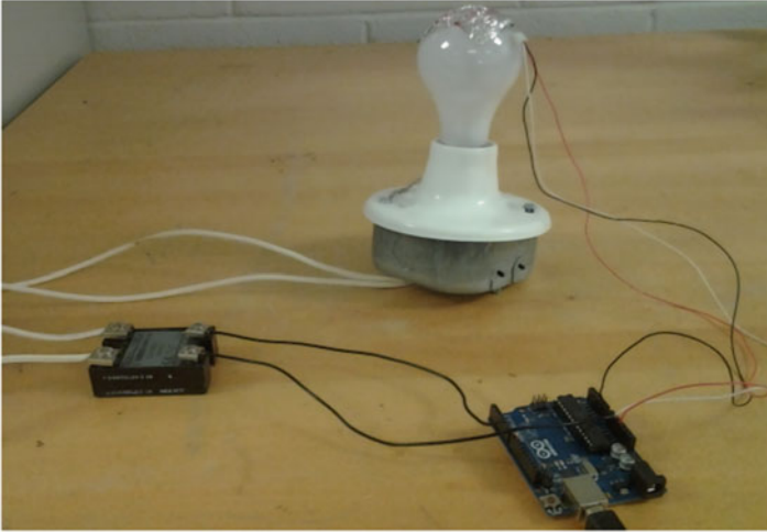
Fig. 12.2 Connection diagram: lightbulb, Relay and Arduino. (Source: Mendoza and Cordero (2018))
