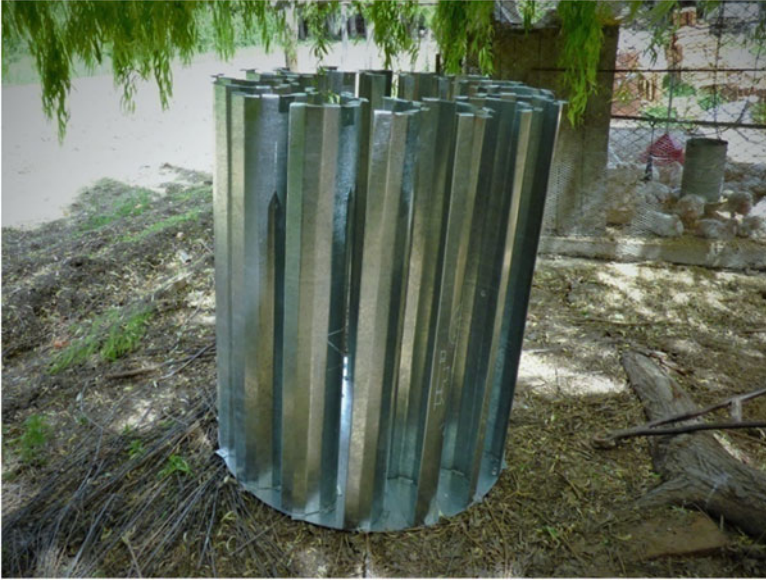
Image 8.2 Another rotor design for Savonius windmill. (Source: Authors' own work)
