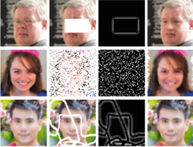
Fig. 3. Baseline DCGAN semantic inpainting model based on [20]. (Left to Right) Original image, input image, importance term and reconstructed image.
