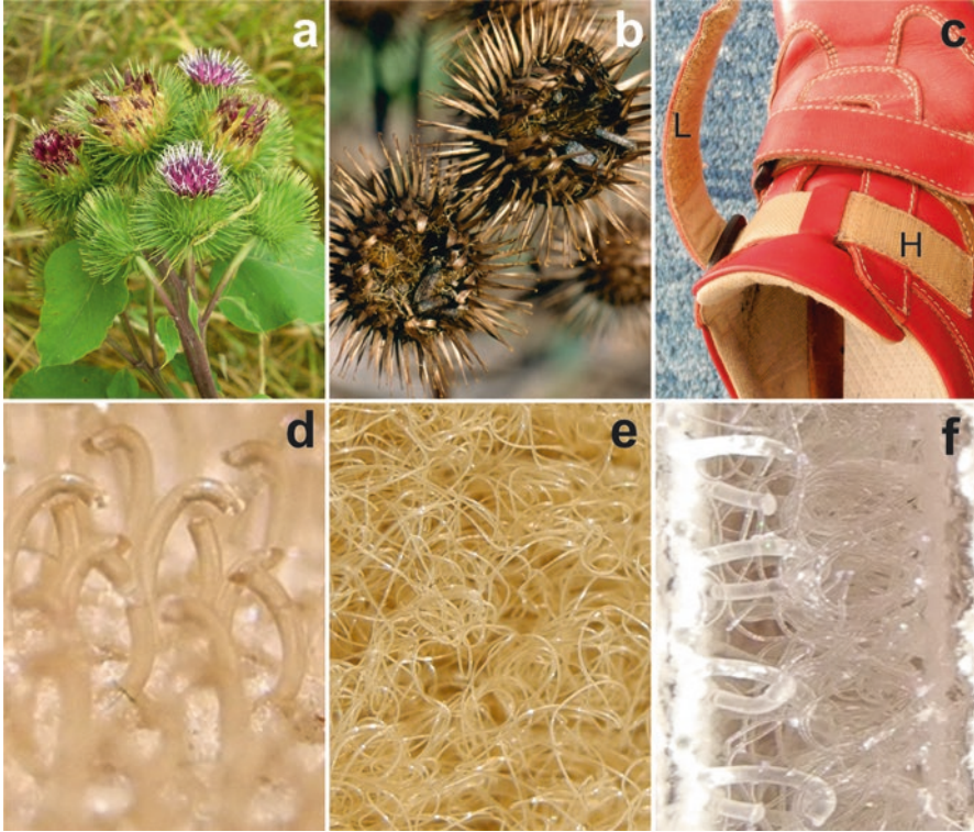
Fig. 3.11 Hook-and-loop fastener (Velcro fastener): model and imitation. (a, b) Inflorescences and infructescences of the greater burdock Arctium lappa . (c) Shoe with Velcro fastener. H hook layer, L loop layer (fine threads). (d) Hooks. (e) Curled threads (loops). (f) Closure of both layers in section. (Image credit: Own photographs)
