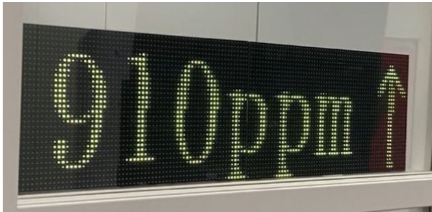
Fig. 8. Risk visualization using an LED matrix array
