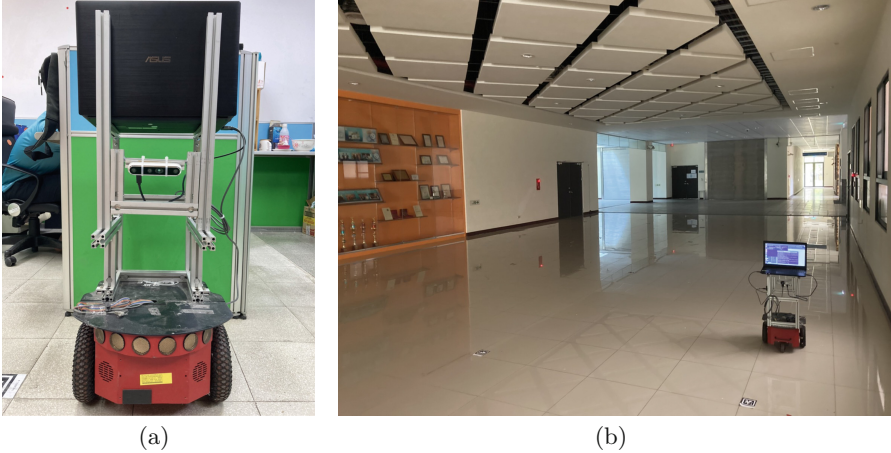
Fig. 5. (a) The mobile robot system constructed for the experiment. (b) The indoor environment used for evaluation in our experiment.
