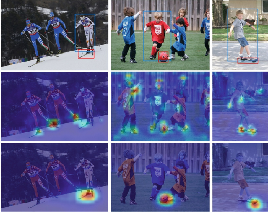
Fig. 10. Comparison of human-centric attention maps obtained by our method vs. iCAN [6], on example images from the V-COCO dataset. The first row contains images with the bounding boxes of the candidate human-object pairs, the second row contains the attention map obtained from the iCAN module, and the third row contains the attention map obtained from the improved iCAN module
