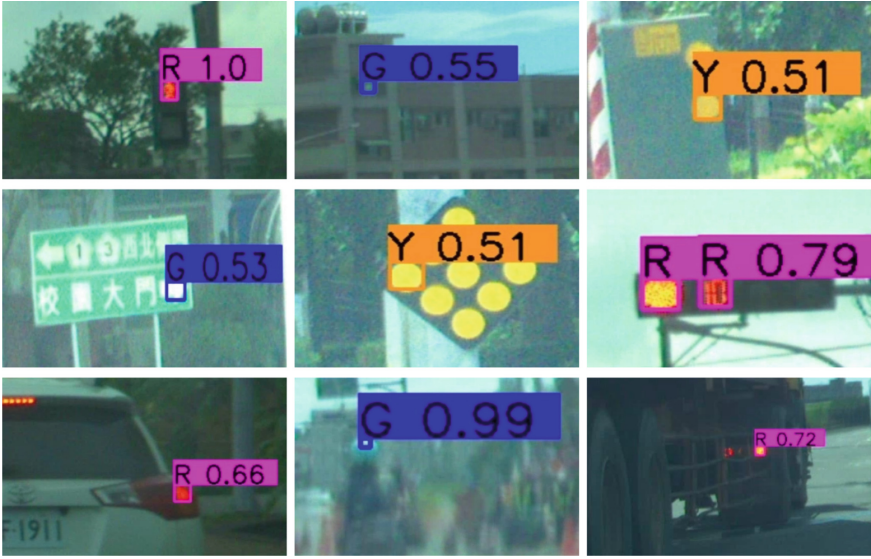
Fig. 5. The false positives frequently obtained in the first stage detection results, including pedestrian lights, brake lights, traffic signs, etc.
