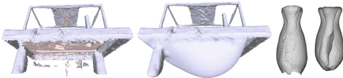
Fig. 10.6 From left to right. (1) bottom of machine frame with artifacts. (2) reconstruction result. (3) scanned model of vase. 4: reconstruction result of vase. Even the inside was reconstructed well, but the mass distribution in the reconstruction result is no longer symmetrical
