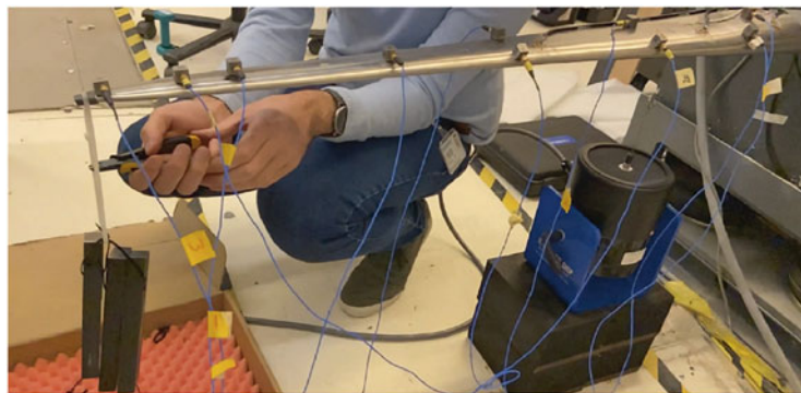
Fig. 4.4 Static load applied at the blade tip during pull and release tests
