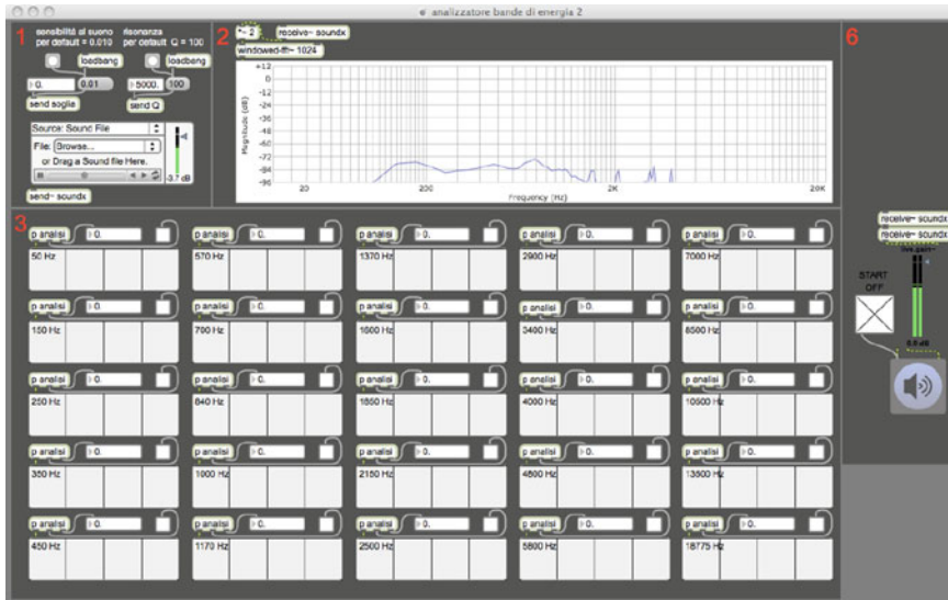
Fig. 19.1 Energy band analyzer. This figure shows the functioning of the patch during the analysis of a live audio sample. The screen is divided into six parts. This image shows part n.1, where the audio is selected; n.2, where the artist can see the live processing of energy; n.6 that is the on and off button; n.3 that shows the live energy progression in each of the 25 bands (which are approximate of 100 Hz each)
