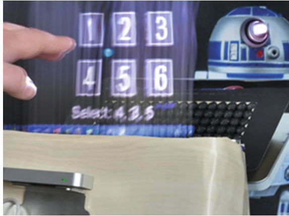
Fig. 6 From front left to back right: leap motion controller, fogscreen, phased ultrasonic 16 \times 8 array, and projector (masked with an R2D2 printout) (Sand et al., 2015a)
