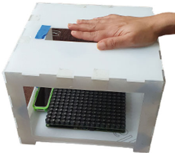
Fig. 4 Experimental setup. It was used during both the practice and test run of the patterns. The large slit allowed the participants to position and rest their hand while exposing their index and middle fingers to the tactile stimulation patterns delivered by the Ultrahaptics device
