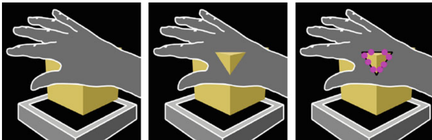
Fig. 1 When a tracked hand touches a virtual object, multiple focal points are generated at the intersection (Long et al. 2014)
