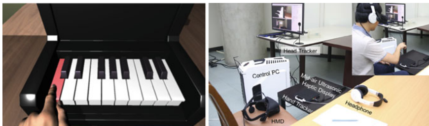
Fig. 2 A VR scene of AirPiano (left) and its setup (right)
