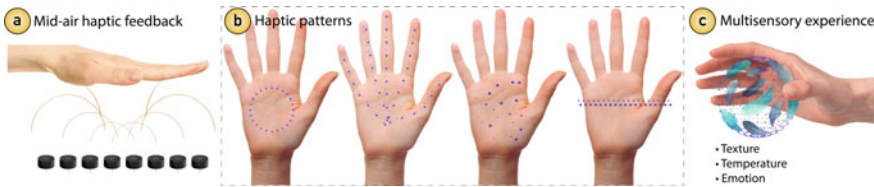
Fig. 2 a Mid-air haptic feedback, b different haptic patterns on the user’s hand, c the associations of the haptic patterns with sensory features can produce a multisensory experience
