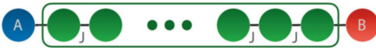
Fig. 6 Alice and Bob have access, respectively, to qubits A and B , located at the two ends of a spin chain (wire). Entanglement between the two qubits can be generated by exploiting the dynamics of the quantum wire, whose Hamiltonian includes a nearest-neighbour interaction term
