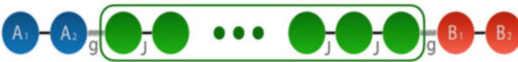
Fig. 7 Alice and Bob have access to qubits A_1, A_2 and B_1, B_2 , respectively, located at the two ends of a spin chain (wire), which is capable of generating an entangled state by exploiting its intrinsic dynamics
