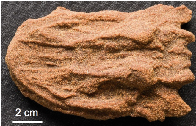
Fig. 2. Example of the 3D printed model, #7 made out of apricot kernel flour.
