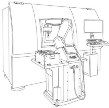
Fig. 1. Schematic image of the tomograph with the supply robot [14].
