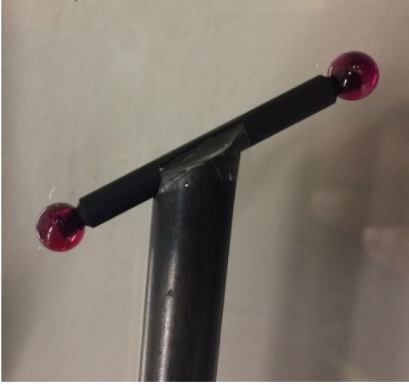
Fig. 2. Test standards used in the study: a) Ball-bar, b) 1, 5, 10 and 20 mm gauge blocks.
