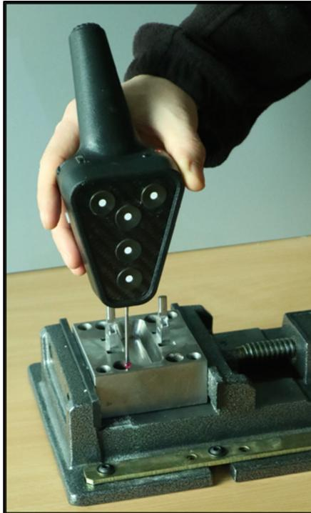
**Fig. 3.** Probe with active markers.
