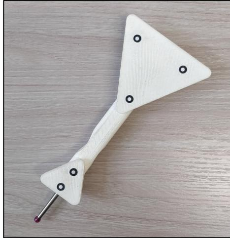
**Fig. 2.** Probe with passive markers.
