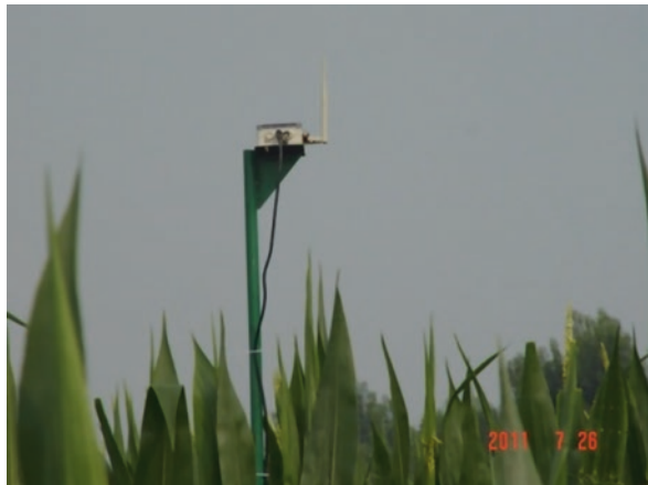
Fig. 2.7 Schematic diagram of the soil moisture monitoring system based on wireless sensor network
