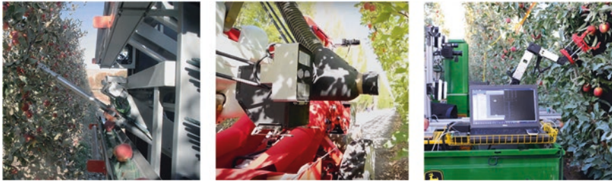
Fig. 12.4 Example of three robotic apple picking systems. From left to right: FFRobotics (multi-layer linear motion with three-finger gripper), Abundant Robotics (parallel robotic arm with vacuum gripper), and Washington State university (serial robotic arm with three finger gripper)
