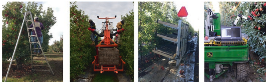
Fig. 12.2 Illustration of the evaluation of tree fruit harvesting methods, from left to right are: manual picking, harvest assist platform, mechanical shake-and-catch, and robotic harvesting
