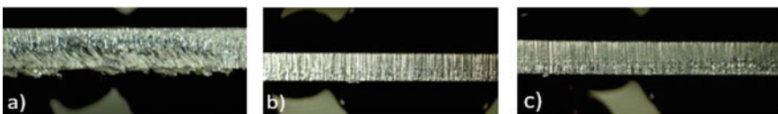
Fig. 9 Cutting edge striation pattern formation at different cutting speeds of 1 mm thickness material, a 2 m/min, b 3 m/min and c 4 m/min [45], (reprinted with permission of Springer Nature, 2021)
