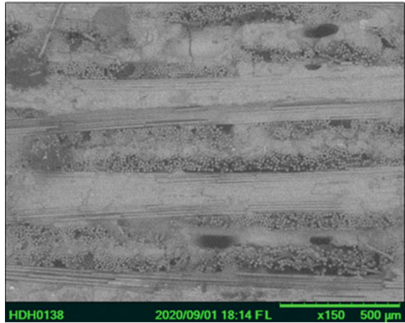
Fig. 1 Image showing the fibre layout of the SiC-SiC CMC
