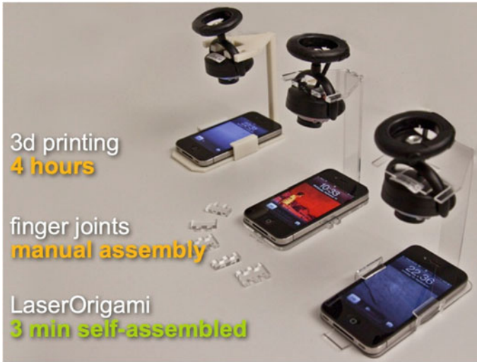
Fig. 18 Advance and commercial application of laser-based forming. Despite 3D printing is an advance solution for making numerous conventional and unconventional objects the time taken to generate origami using laser it takes substantially less time in comparison to 3D printing system
