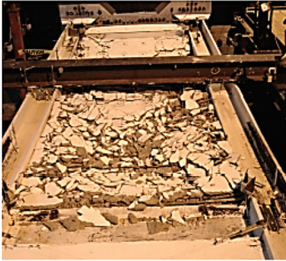
Fig. 17. The composite shear wall at the end of the test and its shear force-drift response [30].
