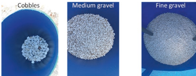
Fig. 15.4 Pictures of the different gravel media during the construction of the pilot STW units
