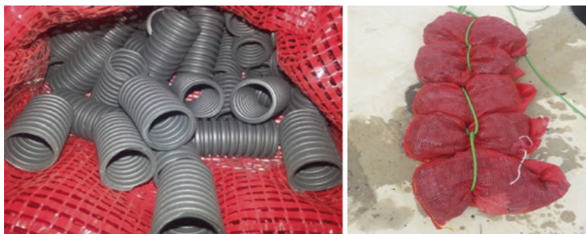
Fig. 11.5 Prepared plastic media (Pieces of conduit in mesh bags)
