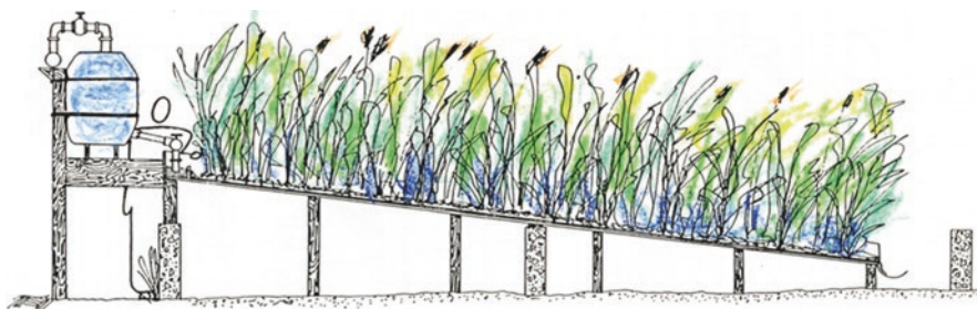
Fig. 5.17 A pilot gravel bed hydroponic wetland at 2% slope tested for heavy metals removal from wastewater [58]
