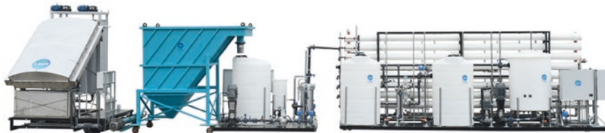
Fig. 1.24 Process equipment of a Livestock Water Recycling (LWR) system [118]
