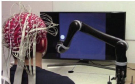
Fig. 4. Brain-computer interface cases: brain-controlled robotic arms from Carnegie Mellon University and the University of Minnesota
