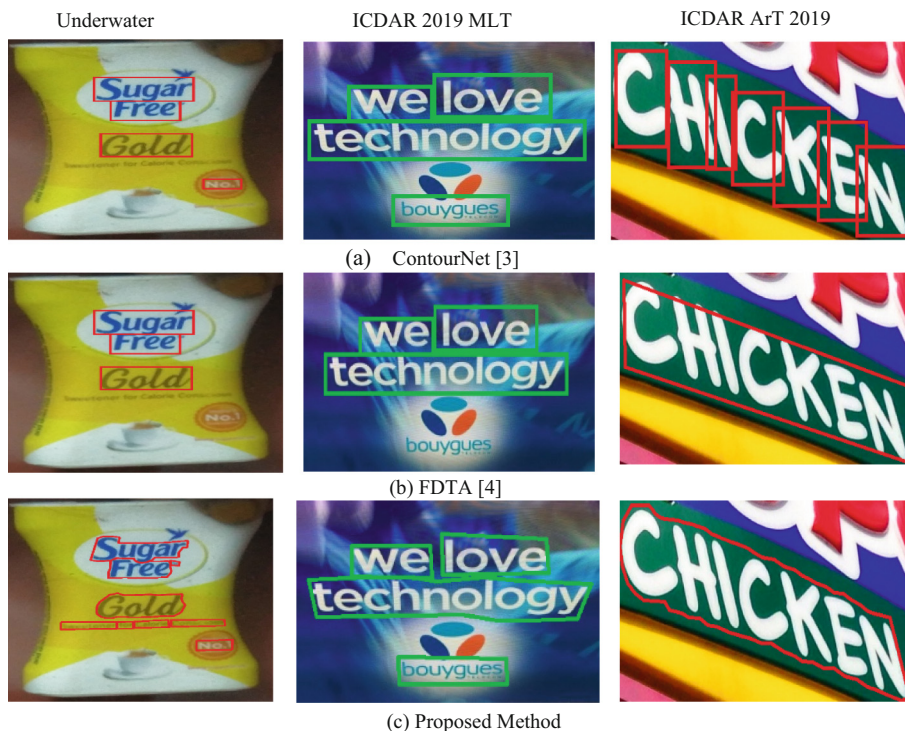
Fig. 1. Example of text detection of proposed and existing methods for under water and natural scene images. Results of ContourNet, FDTA and the proposed method are shown in (a), (b) and (c), respectively.
