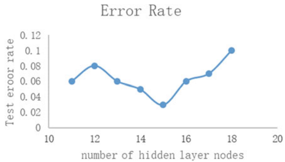
Fig. 4 The variation of error rate with the number of nodes in the hidden layer
