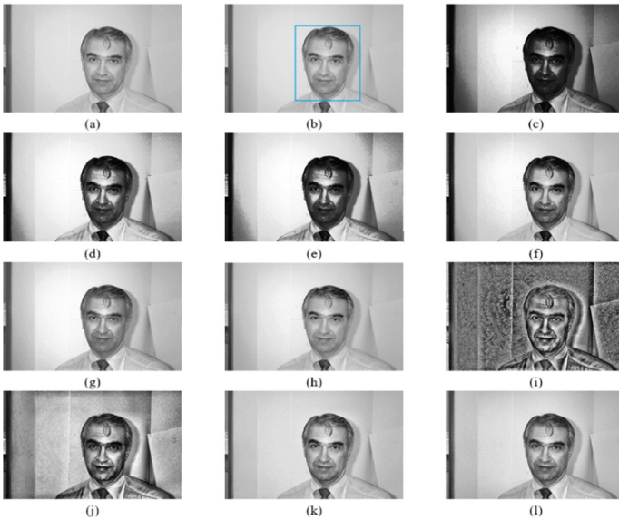
Fig. 2. Visual results for image_0105: (a) Original Image, (b) Important Regions (c) HE, (d) BBHE, (e) DSIHE, (f) RSIHE ( r = 2 ), (g) ESIHE, (h) MVSIHE ( \delta = 0.6 ), (i) AHE ( 63 \times 63 window size), (j) CLAHE (NT = 8 \times 8 , CL = 0.1), (k) MOCS-CLAHE, (l) MOFPAE-CLAHE.
