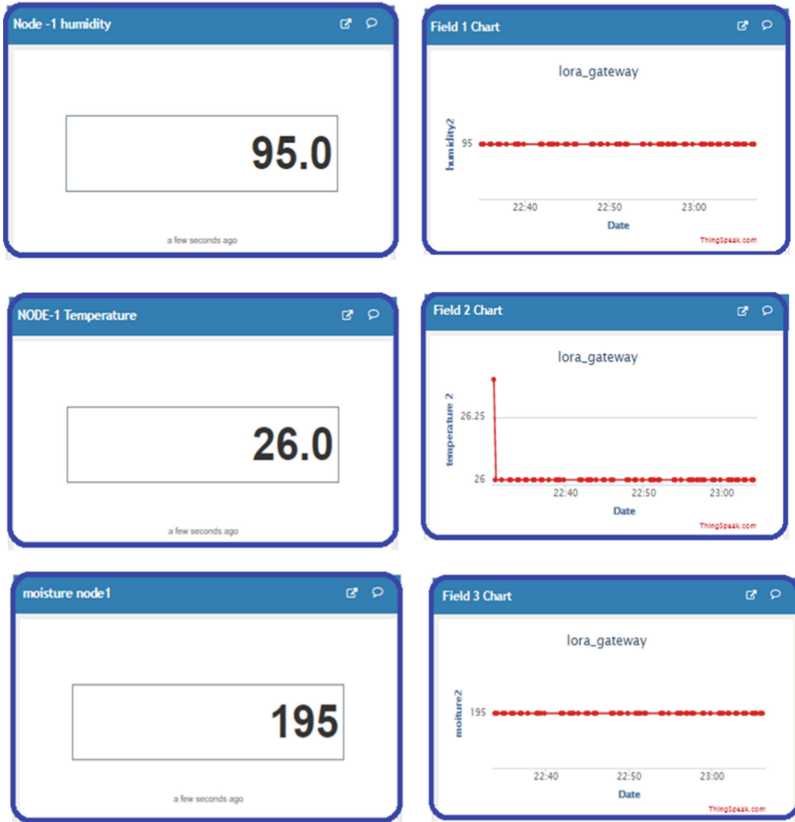
Fig. 7. Visualization of air humidity, temperature, and soil moisture sensor readings pushed on ThingSpeak server.
