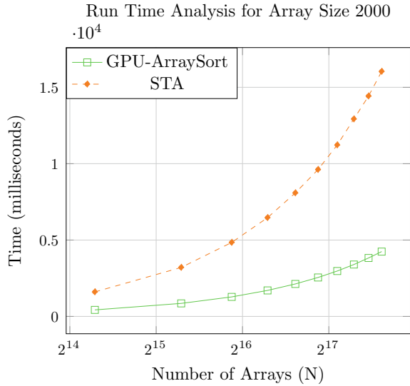
Fig. 7.4 The figure shows time versus number of arrays plots for GPU-ArraySort and the tagged sorting approach using key-based stable sorting algorithm from Thrust library
