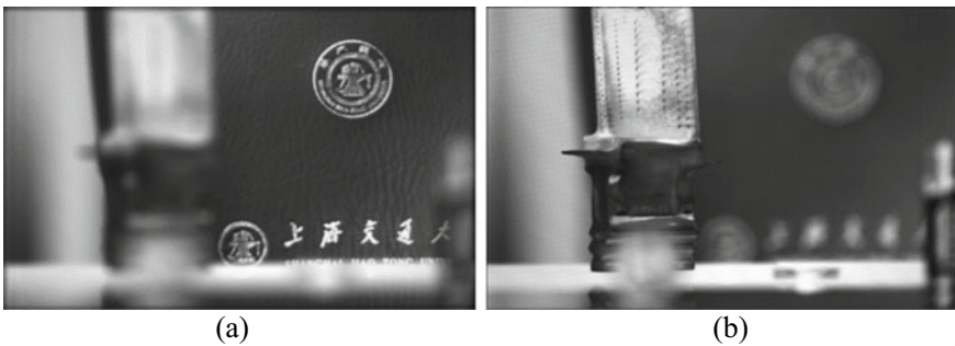
Fig. 2.9 Example of refocused images generated from the raw light-field image shown in Fig. 2.5
